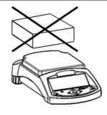
Keep the scales clean. Do not stack material on the scale / balance when it is not in use.
