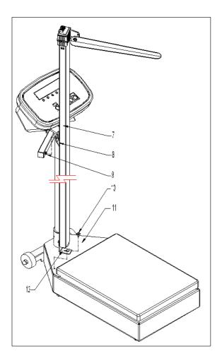
13. Locate the fixing bolt and washer (10) used to secure the height rod to the scale base (11)
