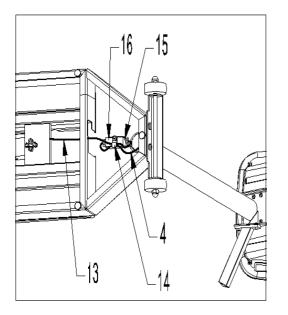
8. Locate the load cell cable (13) ready for connection
