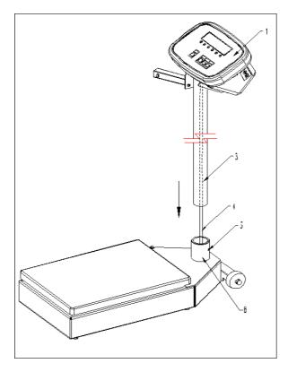
5. Place the cable (4) into the tube support (6) on the scale base.
