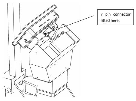
The AE 402 indicator is placed into the mounting bracket, and secured using the two plastic fasteners as shown below:
