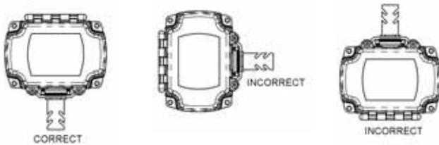
FIGURE 2: OSA Mounting Orientation
