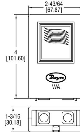
**MODEL WA WATER LEAK DETECTOR** offers affordable and dependable leak detection. This model is ideal for any application where a flood or water leak is likely to occur. It offers a loud audible alarm in the presence of water.
