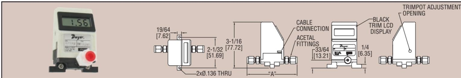
**Series TFP-GI Gas Turbine Flow Meters** are suitable for a wide variety of industrial, commercial, and laboratory flow applications. These meters utilize a turbine wheel and electro-optical detection to convert flow rates into a linear 0 to 5 VDC output signal for recording and data logging. A 3-1/2 digit LCD informs the user of the actual flow rate. A power adapter or mating cable assembly is required for operation.
