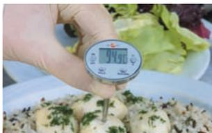
For temperature spot-check measurements in food production
