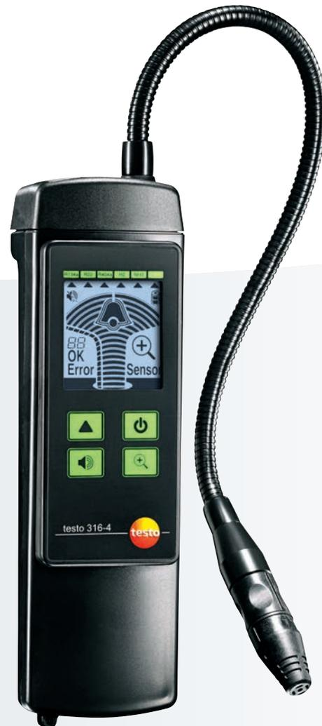
The testo 316-4 (Set 1) is a fast and reliable leakage detector for all common refrigerants. The sensor is permanently monitored and shows malfunctions or contamination in the display. The use of test leaks is thus superfluous. If dirty, the sensor can simply be cleaned, and is immediately ready for use again.
