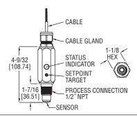
The SERIES TDFS Thermal Flow Switch uses impulse thermal dispersion measurement technique to indicate whether the flow rate is above or below a user set flow rate. It provides NO and NC NPN outputs and two LED, one green and one red for high and low set point indication.
