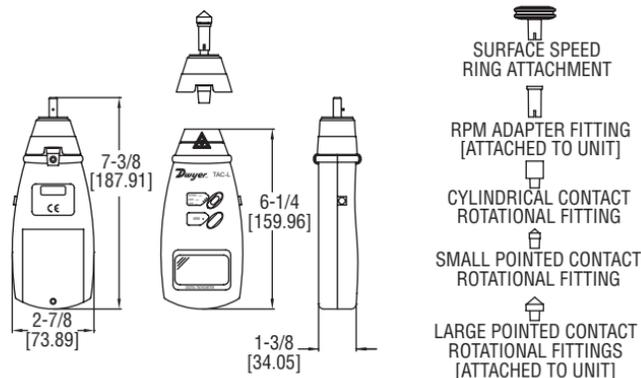
The **MODEL TAC-L** Portable Digital Tachometer measures rotational speed either by contacting a rotatable head to the shaft of the object or by using a photo sensor to detect the reflections from the laser. The housing is made of a strong, lightweight ABS plastic housing, which is designed to comfortably fit in the hand of the user. Supplied with this model are 3 contact rotational heads, a contact surface wheel, and a protective carrying case.
