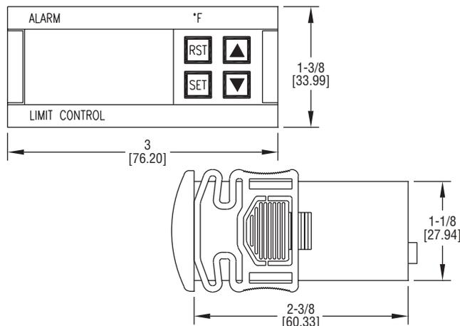
The Series TSF-DF Digital Thermocouple Limit Alarm is a UL approved temperature limit control that provides visual alarm status, along with a 16 amp SPST relay output when a process temperature limit has been reached. After the input temperature returns to normal conditions, the alarm can be either manually or automatically reset depending on how the unit is programmed.
