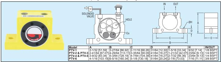
Series PTV Pneumatic Turbine Vibrators are the best choice of high vibration frequency types for a low noise environment. It is usually installed on a vibrating separator, conveyor, automatic arrangement machine, packing machine, or filling machine. The vibration is produced by centrifugal force which arises from the imbalance of movement when compressed air impacts the tangent of the turbine to make it move. The operation noise is low because of ball bearing supports on the running turbine.
