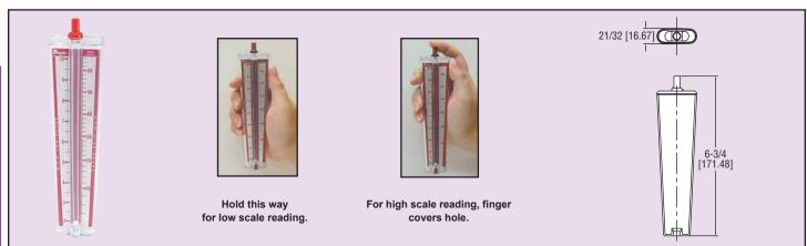
Ideal for yachtsmen, outdoorsmen, farmers, etc. A welcome gift. Use anywhere. Direct reading, no calculations. Hold meter at eye level, back of unit to wind. White ball in tube indicates wind speed. Meter has two scales for max accuracy and easy reading — low, 2 to 10 and high, 4 to 66 mph range. For high range, cover hole with finger. Pocket size, sturdy plastic, has case.
