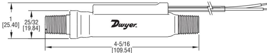
The **SERIES P2** Flow Switches utilize a piston-type design for both air and pure water applications. The switches have preset actuation points from 0.05 to 1.0 GPM for water and 25 CFH to 5 CFM for air. The P2 is comprised of PPE & PS (polyphenylene ether and polystyrene) housing and piston and 316 SS spring and stop pin.
