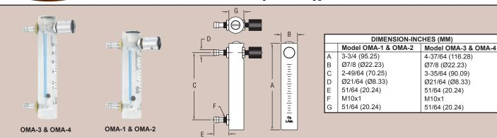
The Compact Series OMA Oxygen Flowmeter is made especially for medical applications and manually controlling flow from oxygen generators. Flow levels are kept stable by precision valve and knob adjustment. The low cost flowmeter is made from durable clear acrylic plastic. The easy-to-read scale is hot stamped into the acrylic so it will not wear off. The ball float is highly visible against the light blue background. Readings are repeatable within  $\pm 4\%$  full-scale accuracy.
