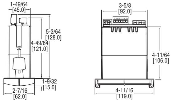
The Series PM's are a series of 1/8 DIN digital panel meters engineered to take in multiple inputs from a variety of instrumentation for the purpose of displaying or controlling a process parameter.
