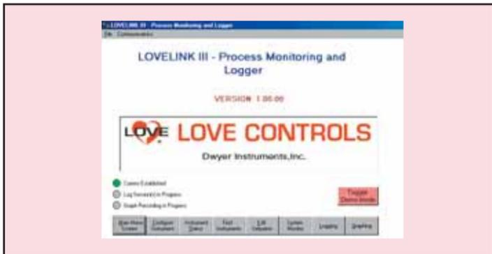
**LoveLink™III** Data Acquisition and Logging Software is the second generation of data acquisition software from Love Controls. This easy to use program allows connection of up to 40 controls on a single computer port. Data logging can be set up by individual control with varying logging periods. LoveLink™III Software is compatible with all Love Controls 2600, 8600, 16A, 16L, 16S, 32A, and 32DZ Series controls.
