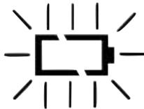
Battery Exhausted: measurements are not possible. When the low battery icon indicates the battery is low, the batteries should be replaced immediately with AAA, 1.5V batteries using the below steps.
