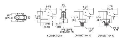
Series A7 Mini Pressure Switches have been designed for high current applications. These switches are small and inexpensive, making them ideal for OEM use. The Series A7 switches utilize a high-quality snap-action switch, which is diaphragm actuated. They have a silicone diaphragm and nylon housing. The A7 switches are compact and lightweight which adds to the ease of installation. The set point must be factory set, but a broad operating range makes them great for a variety of applications.
