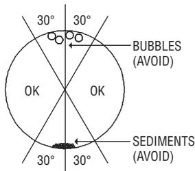
FIGURE 2: Mounting Orientation
