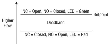
FIGURE 1: Switch Setpoint & Deadband
