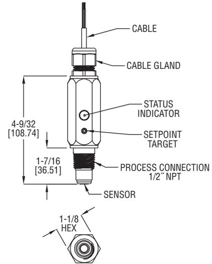
The Series TDFS is a thermal flow switch that indicates whether the flow rate is above or below a user set flow rate. The unit incorporates two LED status indicators providing visual switch indication. The set flow rate (setpoint) is field adjustable and the unit has both NO and NC NPN outputs. See Figure 1 for output and LED actions on change of flow.
