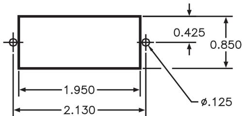
**FIGURE 2-4 CUTOUT DIMENSIONS FOR LCD PANEL MOUNTING**
