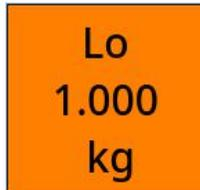
When the weight or quantity value is more than the Lo value, but less than Hi VALUE, the OK box glows green.
