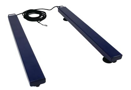
AELP pallet beams provide an affordable solution to weigh oversized or bulky items. Equipped with rugged built-in wheels and handles, AELP pallet beams are easy to set up and move. The low-profile beams permit easy accessibility to simplify loading, weighing and unloading. AELP comes with a 15-foot/5-meter shielded cable, allowing the indicator and beams to be positioned as needed. Four OIML-approved load cells provide precise, consistent measurements.
