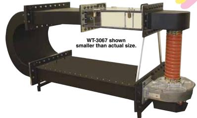
flows up to 50 m/s (10,000 ft/min) using orifice plates (available custom). The clear polycarbonate test section lets the user view the test specimen and allows for flow visualization.
