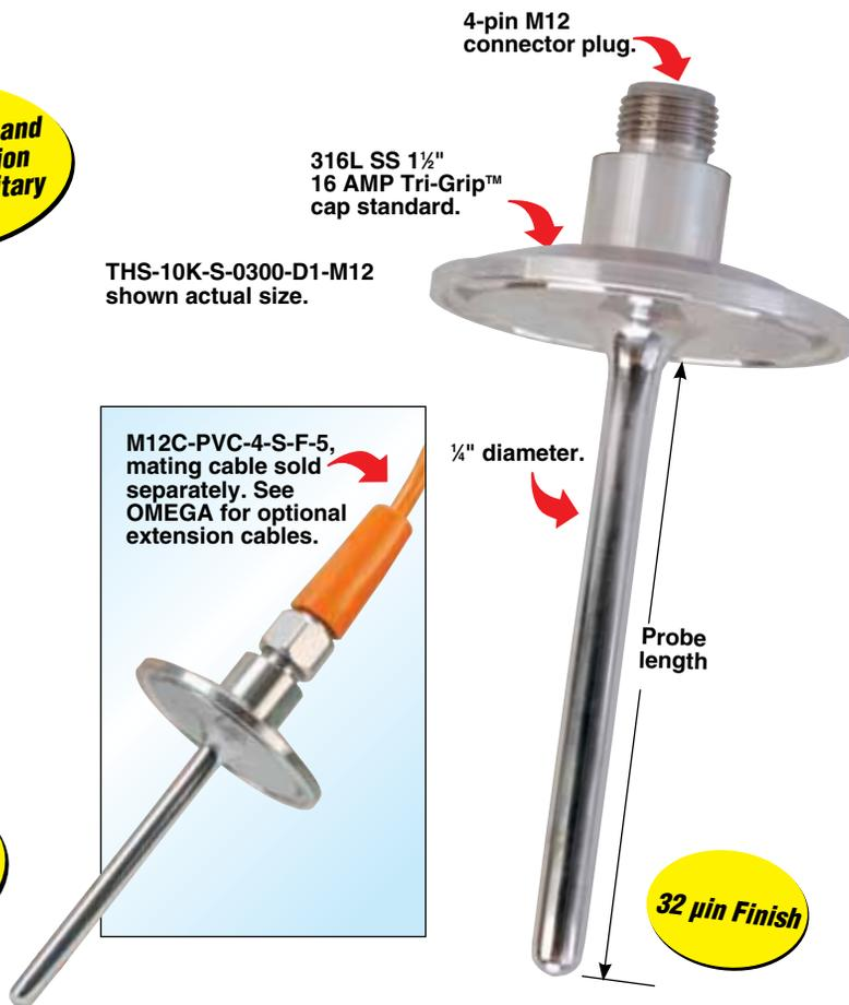
The OMEGA® THS-S-M12 Series thermistor probe assemblies are available in standard lengths from 3 to 6", with standard 10 kΩ (44006) thermistor element. Standard features include a 1 1/2" 16 AMP Tri-Grip™ fitting and a 4-pin M12 male connector termination. Please consult sales for available options, including element types and curves, probe lengths, protection heads and curves, and sanitary fitting styles.
