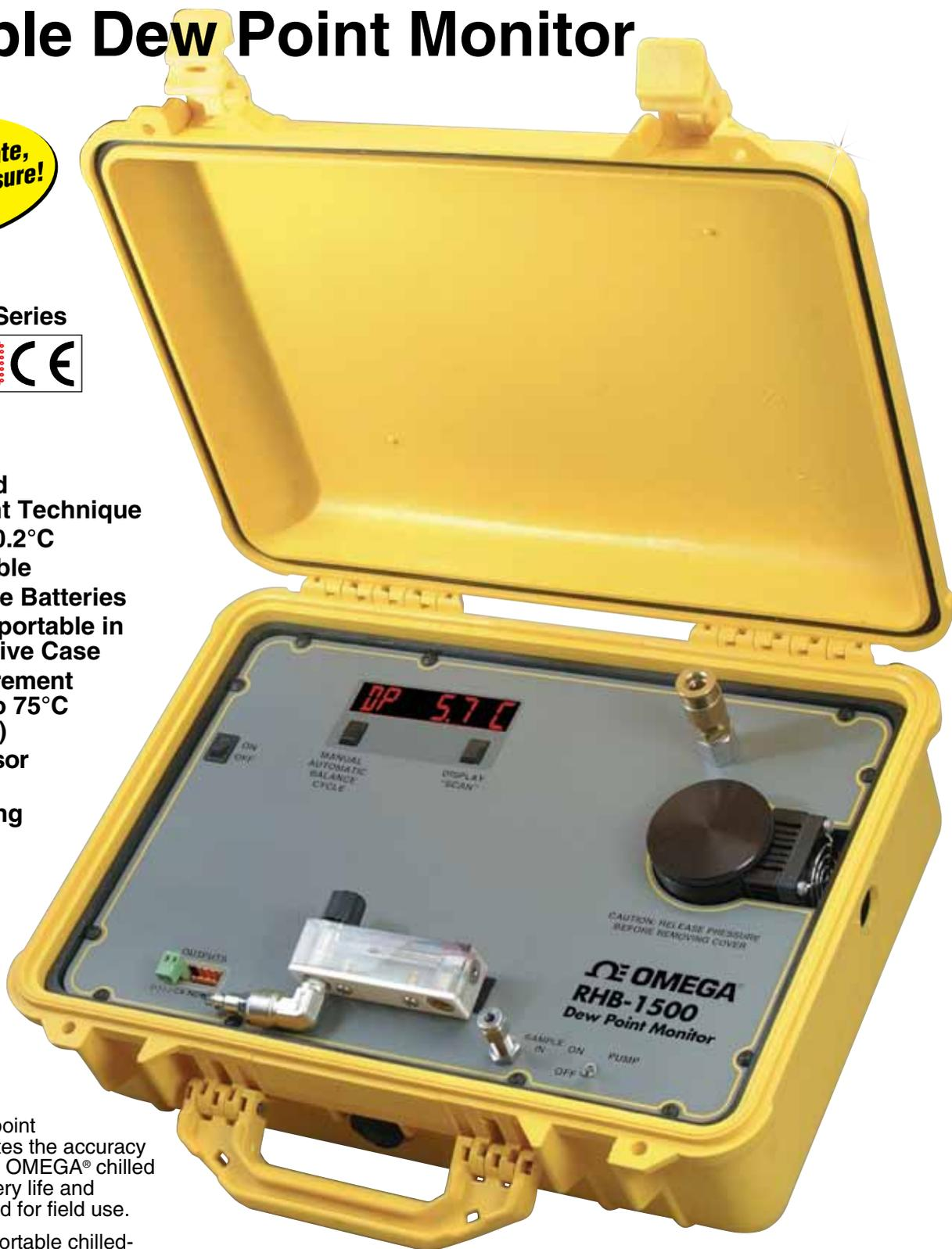
This portable dew point hygrometer integrates the accuracy and reliability of the OMEGA® chilled mirror with the battery life and ruggedness required for field use.
