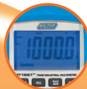
40 000 Count Backlight Display with 41 segmented bargraph
