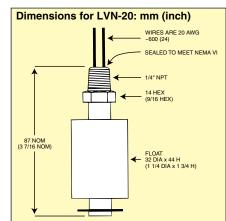
**Switch Actuation:** Approximately ½ the distance from the end of stem to mounting or halfway point of float travel
