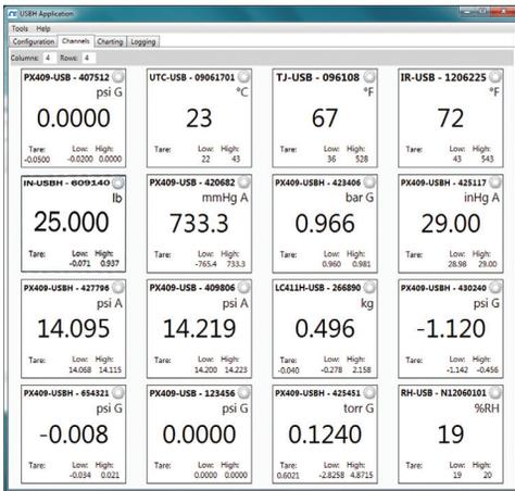
**Channels Window** – Display data from all of your sensors simultaneously. Each channel has configurable user alarms, three data filters, tare, resettable low/high indication, and sample rates ranging from 30 minutes to 1000 Hz.
