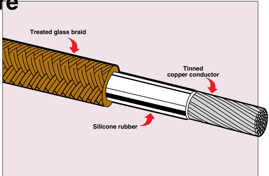
Braided silicone rubber insulated high-temperature lead wires are well suited for use as the exposed leads in appliances and lighting fixtures. HTRG Series wire is also used for range top burners and back panels, steam irons, toasters, broiler ovens, gas dryers, kilns, recessed lighting fixtures and similar applications up to 200°C (392°F).
