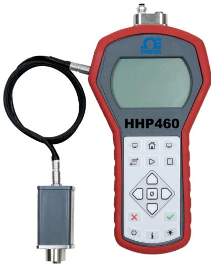
The HHP400 is a portable pressure instrument that offers flexible features to help meet the demand of your everyday pressure measurement needs. This smart manometer can document up to 240 readings in over 30 engineering units. It also has several features including MIN/MAX capture, adjustable damping rates, and auto shut-off. The HHP400 features NIST traceable accuracy up to  $\pm 0.025\%$  of full-scale.
