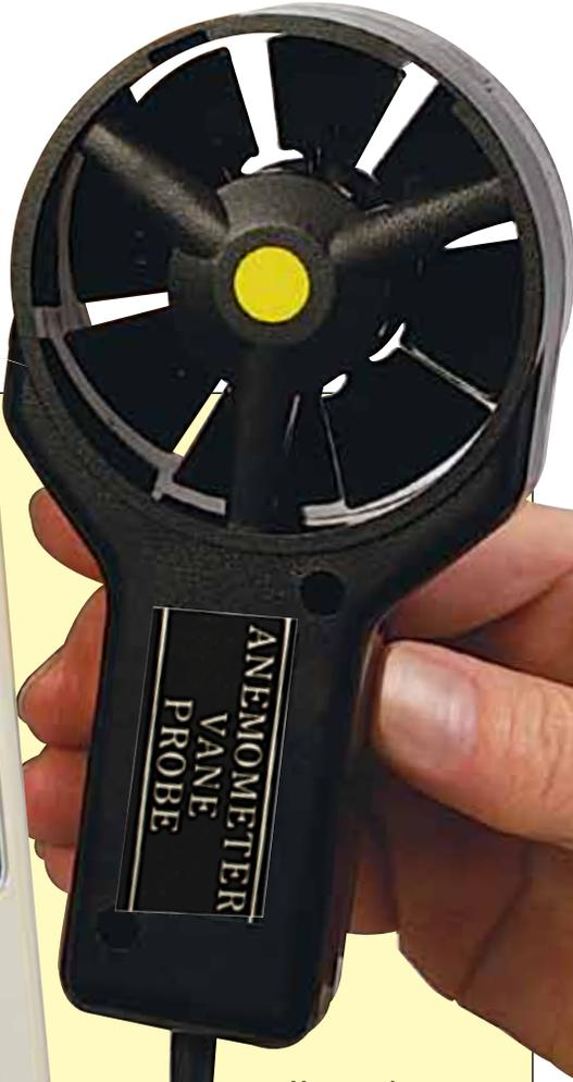
The OMEGA® HHF-SD2 combination vane and standard thermistor anemometer with SD card data logger has multiple features that make it suitable to use in such applications as air conditioning and heating systems, measuring air velocities and wind temperature. What sets the HHF-SD2 apart from other vane anemometers is that it incorporates a real-time SD card data logger.
