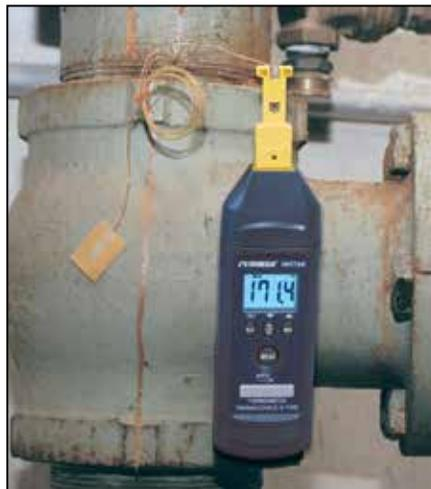
HH74K shown with optional SA1-K-SC, self-adhesive thermocouple.
