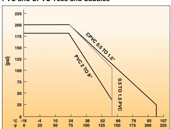
**WARNING:** THE ABOVE PRESSURE/TEMPERATURE CURVES ARE SPECIFICALLY FOR THE FP-5100. FP-5300, AND FP-8500 SENSORS. DURING SYSTEM DESIGN, THE SPECIFICATIONS OF ALL COMPONENTS MUST BE CONSIDERED. IN A METAL PIPING SYSTEM, A PLASTIC SENSOR WILL REDUCE THE SYSTEM SPEC. ON THE OTHER HAND, IF USING A PVDF SENSOR IN A PVC PIPING SYSTEM, THE FITTING WILL REDUCE THE SYSTEM SPEC.
