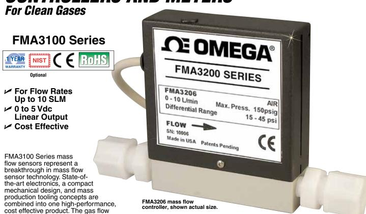
Using the basic FMA3100 thermal mass flow sensor, the FMA3200 mass flow controllers offer accurate, stable control of gas flows in a compact package. In power-off mode, the flow control valve is closed with a minimal leak rate. This cost-effective controller is ideal for many OEM applications, with a 0 to 5 Vdc linear output and a 0 to 5 Vdc control input.
