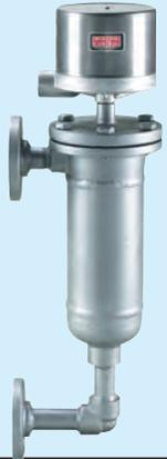
Series 214 has two vertical flanges (1" RF forged steel - ANSI specifications). Flange centerline 15 5/8" (403 mm). Other centerlines available.
