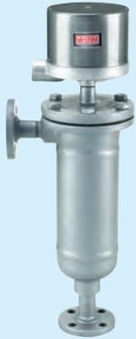
Series 213 has one vertical and one horizontal flanged connection (1" RF forged steel - ANSI specifications). Flange centerline 15 1/4" (387 mm). Other centerlines available.
