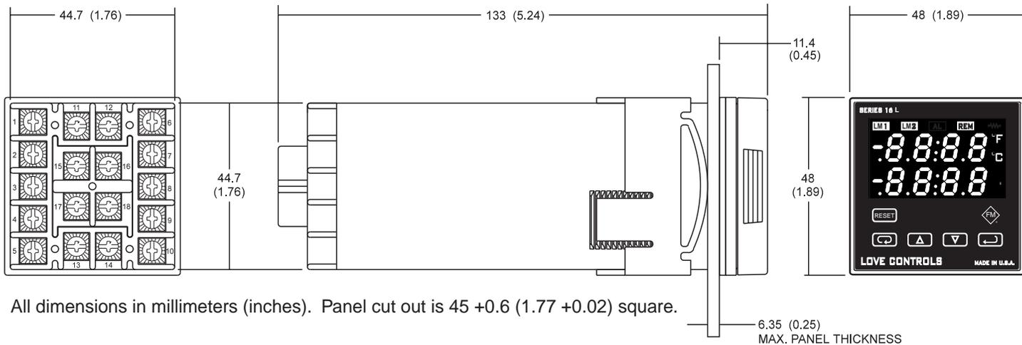
All dimensions in millimeters (inches). Panel cut out is  $45 \pm 0.6$  ( $1.77 \pm 0.02$ ) square.
