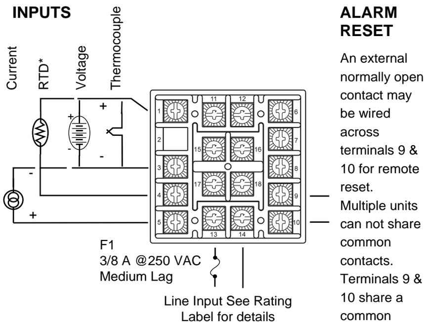
\* For 2-wire RTD use terminals 1 & 3, and place a jumper wire between terminals 3 & 4.
