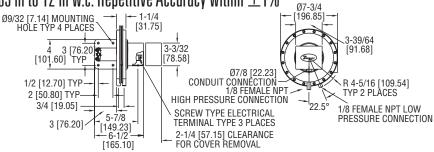
On the SERIES 1630 our highest precision conventional large diaphragm pressure switch provides maximum dependability. In addition, it incorporates a visible set point indicator for maximum convenience. UL and CSA listed, FM approved for general service. Electrical capability of 15 amps handles most small electrical loads. For use only with air or compatible gases.
