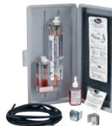
104, solid plastic portable vertical manometer shown attached to inside of carrying case cover. Gage may also be removed from case and used in standing position or attached to any vertical steel surface with magnetic clips provided.
